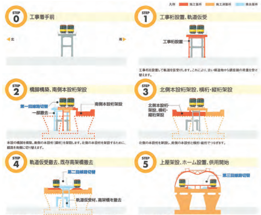
駅移設概略施工ステップ Steps (simplified for clarity) for station relocation
